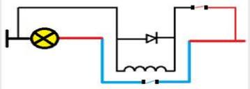
The image below shows the sub-circuit through the diode when the current through the winding is switched off.
