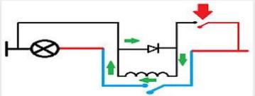
The image below shows the winding being short circuit by an incorrectly fitted diode. Not the orientation of the component.
